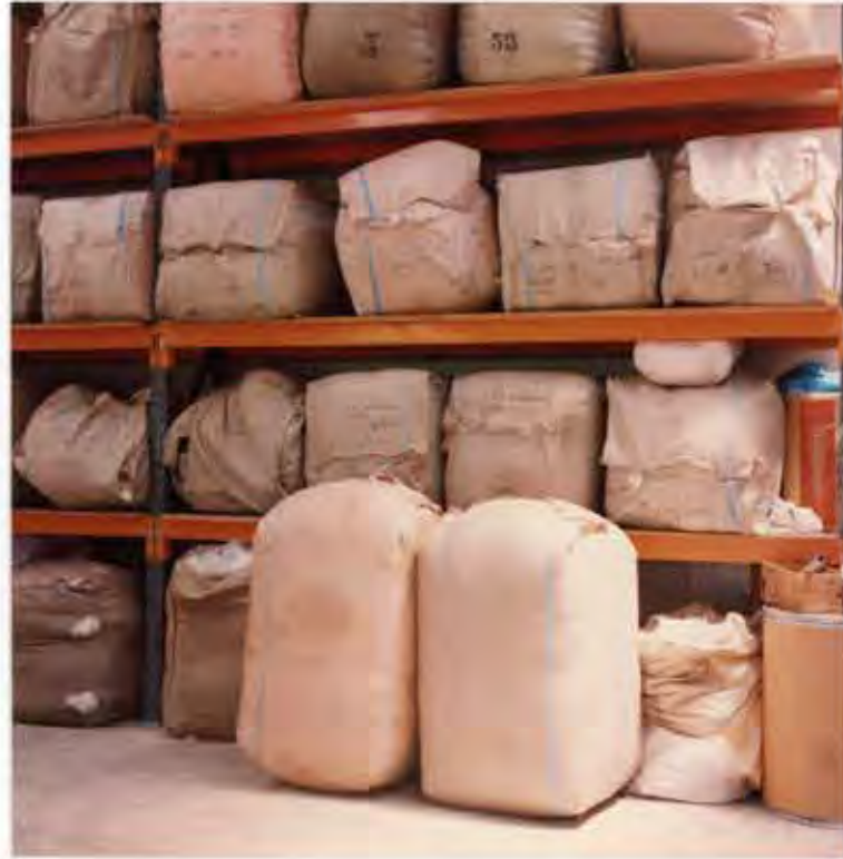
Bales containing wool samples used to calibrate various equipment.
