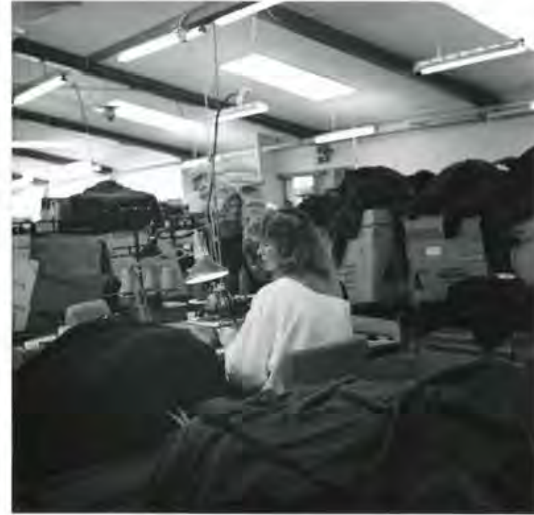
Woman at work at Tamahine Knitting. The company uses a piecework payment system. As part of its quality control, any faults discovered along the line must be corrected by the previous person to work on the item.
