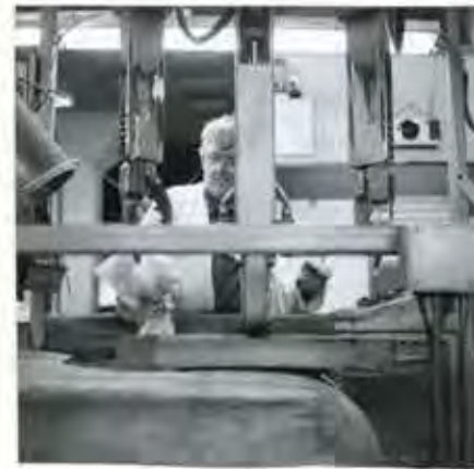
Coring machine takes samples to be tested.
