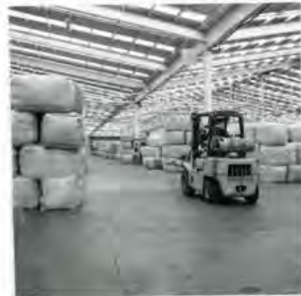
A particular lot can be located by the row number and area where it has been placed. The markings on the bales indicate the farm, lot number, and number of bales in the lot. At this stage, a typical bale weighs 160-180 kg (350-400 lbs).
