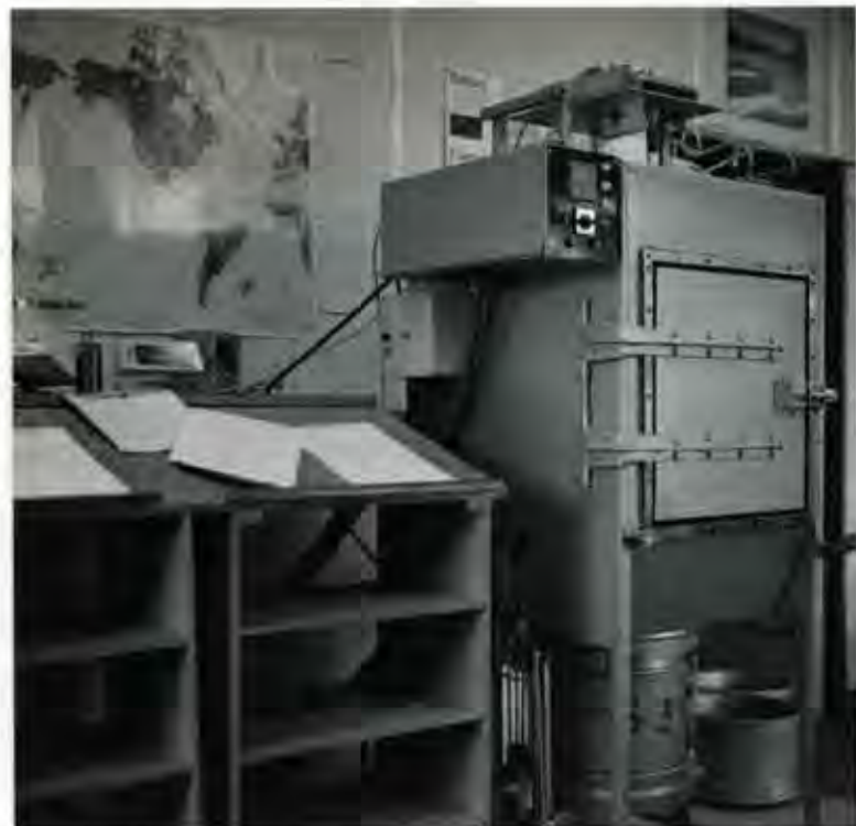
Custom-built oven at the NZWTA branch office on Portsmouth Drive, Dunedin is used to dry wool in order to determine regain. Regain is a percentage figure which is used to correct the weight of a consignment for changes caused by moisture.
