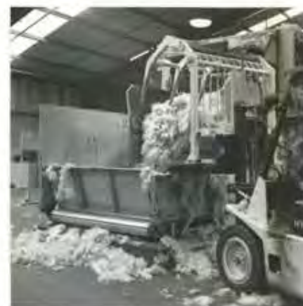
Wool is fed into the scouring machine...
