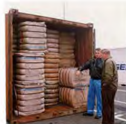
Port workers discussing what to do with a container that has been stuffed so full that its sides bulged out. Some firms have less modern presses and may have to use a tractor to shut the door.
