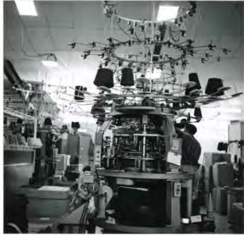
Circular machine for knitting jerseys at Tamahine Knitting Co. Limited off Kaikorai Valley Road in Dunedin. The company also has computerized long-bed machines. CAD will soon allow Tamahine to scan photos and produce patterns with up to 27 colors.
